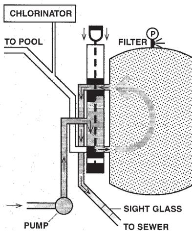
**Figure 12-7** The backwash cycle. The backwash valve has the capability to reverse the flow of water through the filter. When backwashing is in operation, water does not return to the pool but is pumped to the sewer, passing the sight glass. Backwash continues until the water passing the sight glass is clear.
