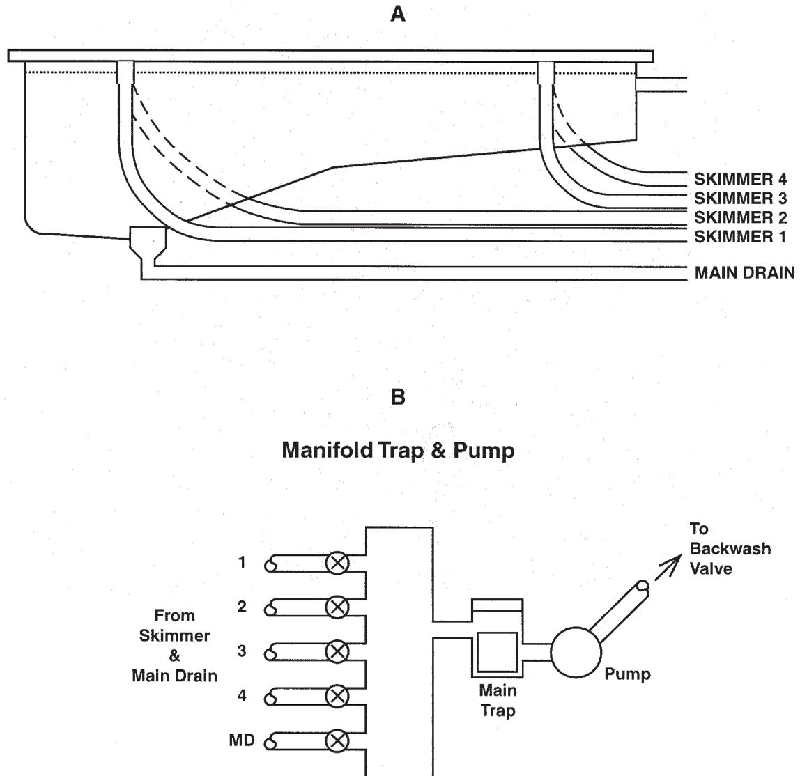
**Figure 12-2** (A) Profile view of pool shows shallow and deep ends of pool with plumbing for *main drain* and 4 skimmer lines. (B) Water from these 5 lines is collected in a manifold with regulating valves on each line to control the flow of water. Water is then collected and sent through the *main trap*. This trap should be opened periodically, and the basket removed and emptied. Water is then drawn into the pump due to vacuum pressure from the pump when it is running.
