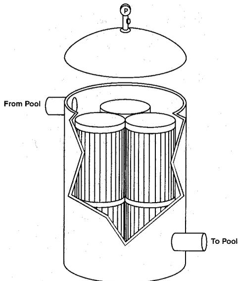
**Figure 12-6** A cartridge filter usually contains 6 cartridges, as shown. The water surrounds each cartridge, made of heavy filter paper, and is forced through the filter to the inside. Water is then collected at the bottom of the filter and returned to the pool. The filters must be opened periodically and the cartridges removed, hosed off, and acid washed.
