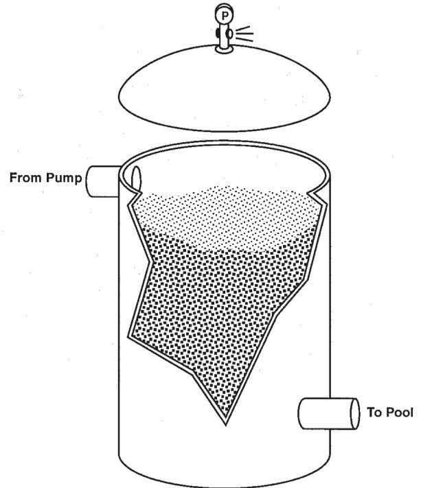
**Figure 12-4** After passing the backwash valve, water enters the filter. The filter shown is an earth sand (ES) filter. Water enters the top and is forced down through the filter under pressure. Water is then returned through a heater (if present), a chlorinator, and finally to the pool under pressure.
