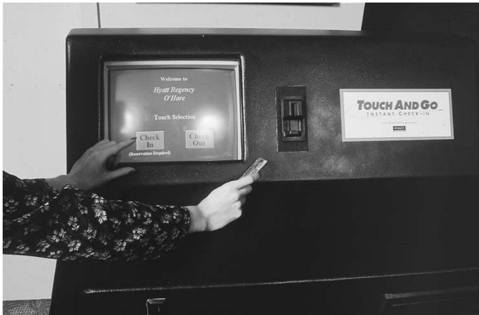
Figure 7-20. A guest may choose to use the self-check-in option of a property management system. The process is initiated with a credit card. (Photo courtesy of Hyatt Hotels and Resorts.)
