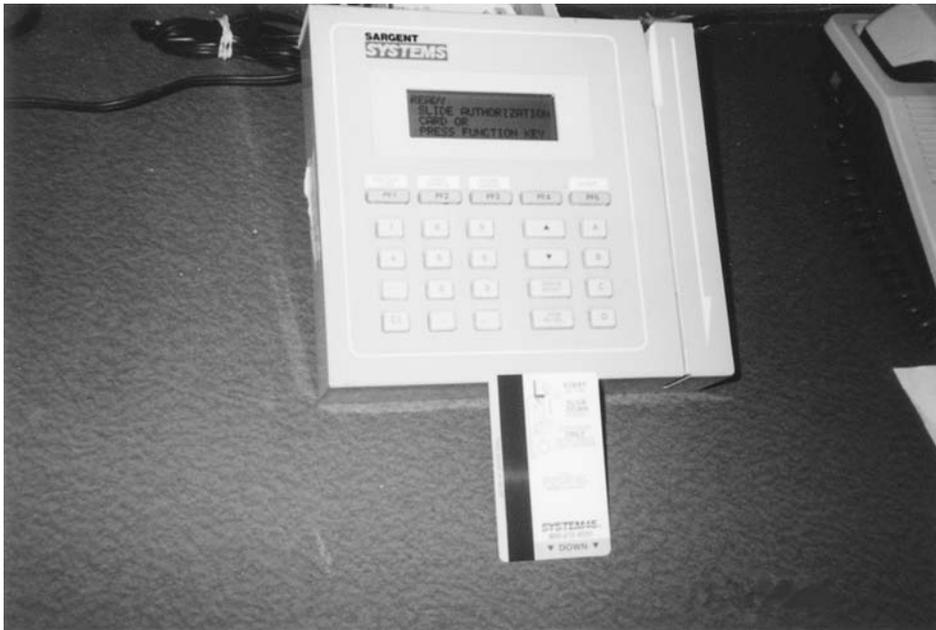
**Figure 7-14.** *An electronic device is used to prepare new electronic room keys for guests. (Photo courtesy of Lincoln Plaza Hotel and Conference Center, Reading, Pennsylvania.)*
