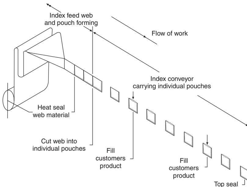
**Fig. 7.5** Horizontal form/fill/seal sachet/pouch machine.
