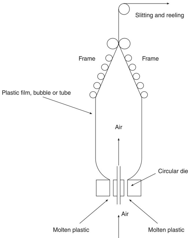
**Fig. 7.3** Blown film manufacture.
