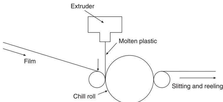
**Fig. 7.14** Extrusion coating of plastic film.
