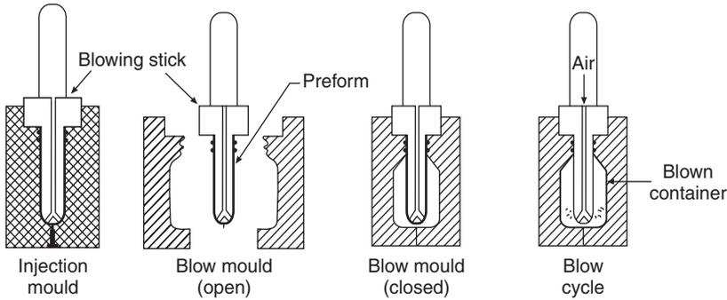
**Fig. 7.9** Injection blow moulding. (Courtesy of The Packaging Society.)
