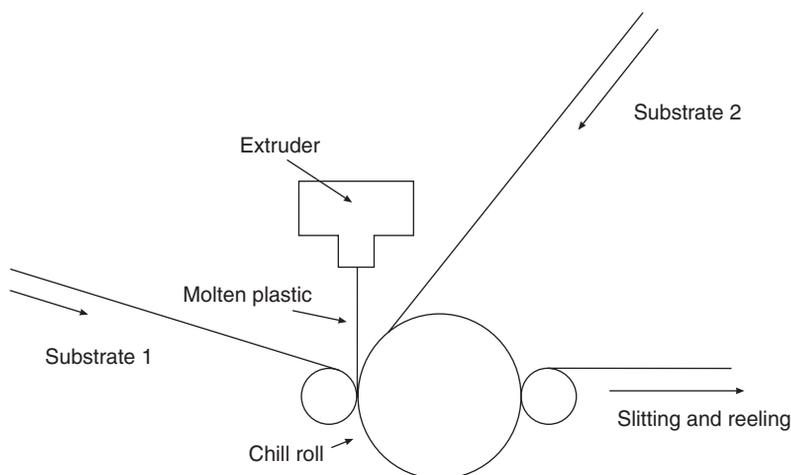
**Fig. 7.15** Extrusion lamination.
