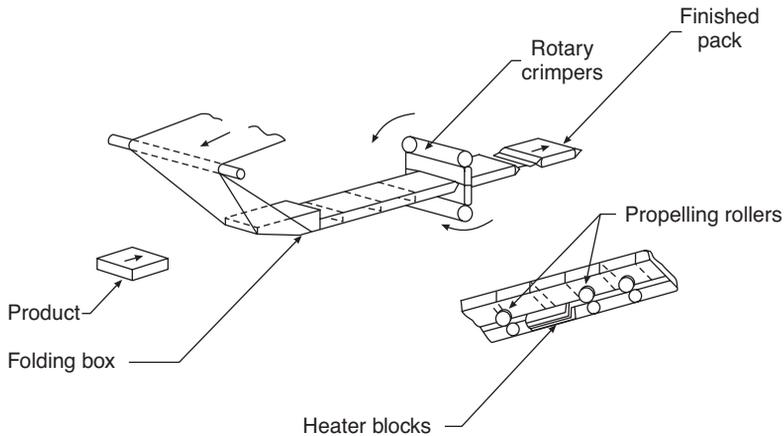
**Fig. 7.7** Horizontal form/fill/seal (f/f/s), flowpack type machine.
