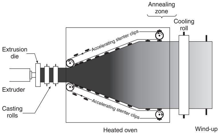
**Fig. 7.4** TD orientation by Steiner and MD orientation by acceleration in machine direction. (Courtesy of The Packaging Society.)
