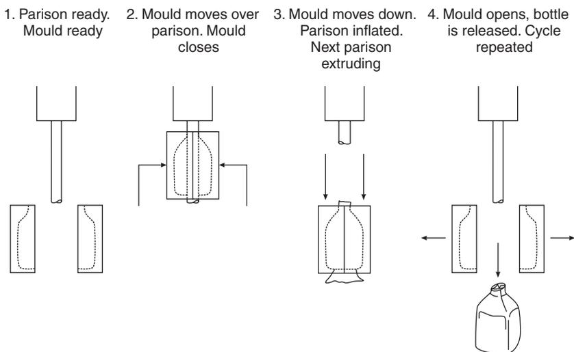
**Fig. 7.8** Extrusion blow moulding. (Courtesy of The Packaging Society.)
