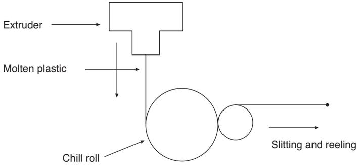
**Fig. 7.2** Production of cast film.
