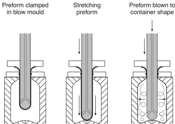
**Fig. 7.10** Stretch blow moulding – applicable to both extrusion and injection blow moulding. (Courtesy of The Packaging Society.)
