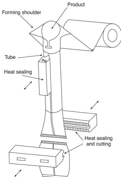
**Fig. 7.6** Vertical form/fill/seal (f/f/s) machine.
