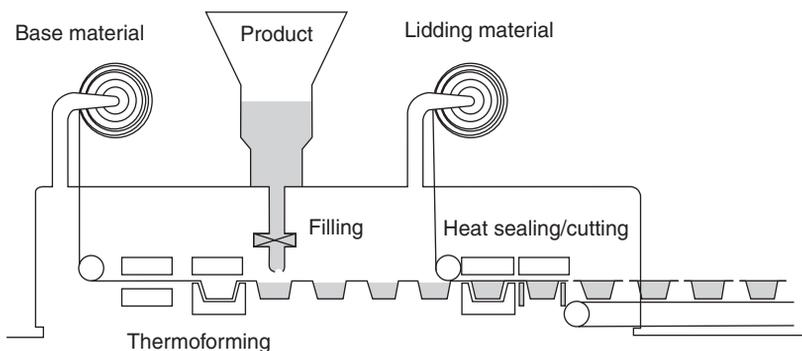
**Fig. 7.12** Thermoforming, filling and sealing.
