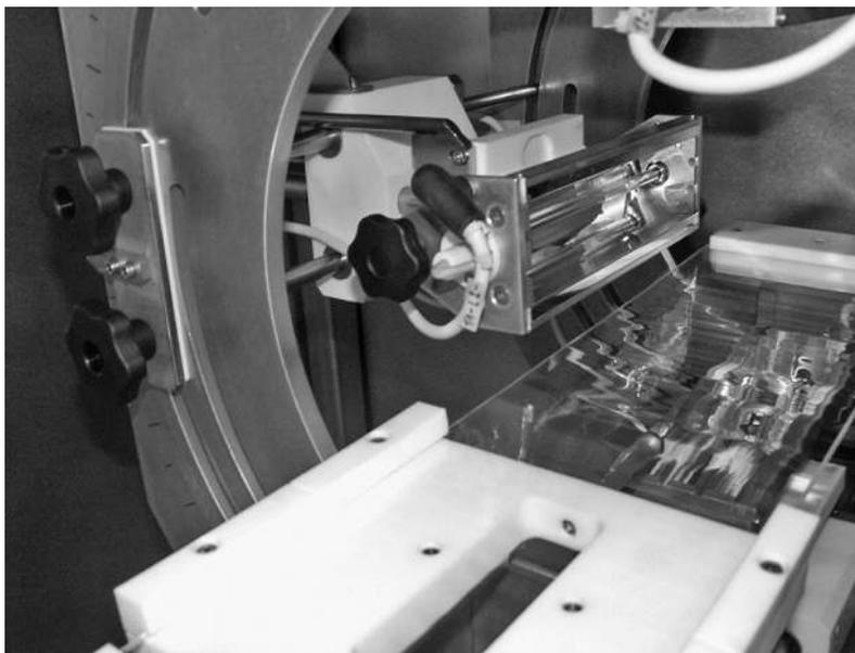
**Fig. 2.9** Pilot pulsed light equipment for surface decontamination. (Courtesy of Claranor.) (For a colour version of this figure, see Plate 2.9.)
