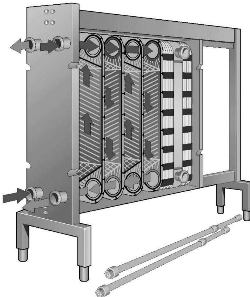
**Fig. 2.6** Plate heat exchanger for processing thin liquids. (Courtesy of Tetra Pak.).
