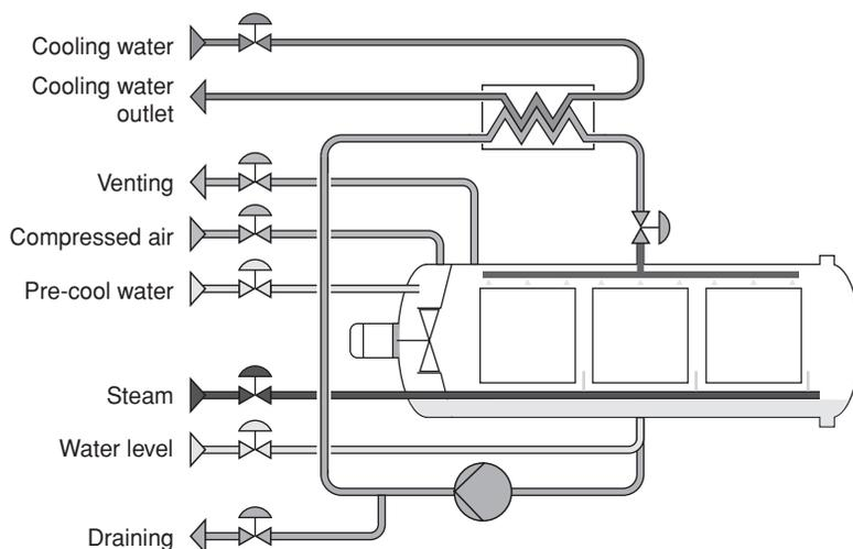
**Fig. 2.2** Example of a batch retort operating on the steam and air principle. (Courtesy of Lagarde.) (For a colour version of this figure, see Plate 2.2.)
