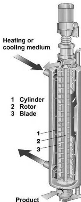
**Fig. 2.8** Scraped surface heat exchanger for processing medium and high viscosity liquids, including those with particulates. (Courtesy of Tetra Pak.)
