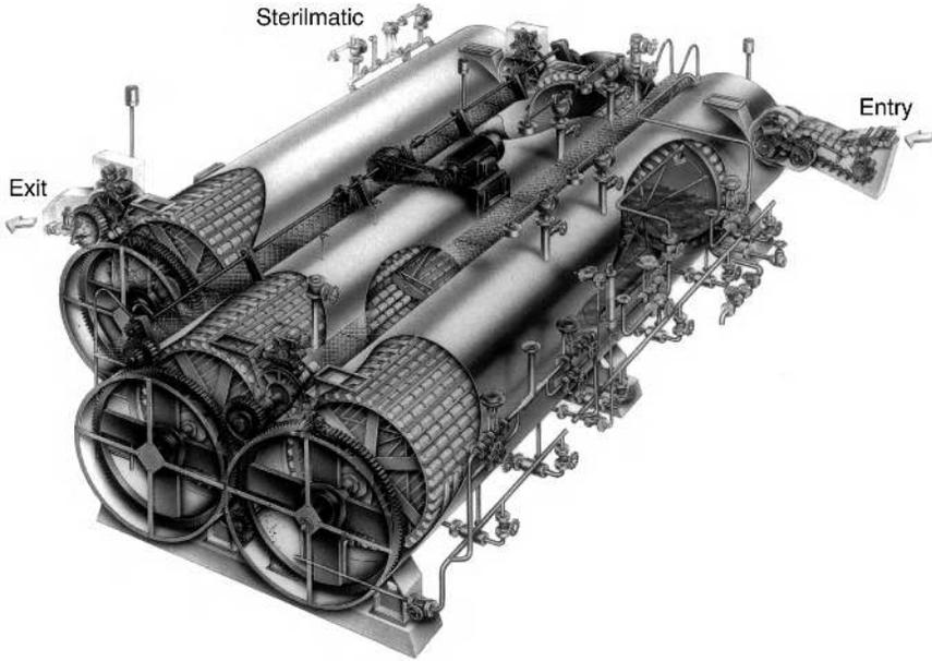
**Fig. 2.4** Reel and spiral cooker-cooler for processing cylindrical food cans. (Courtesy of JBT FoodTech, formerly known as FMC FoodTech.)
