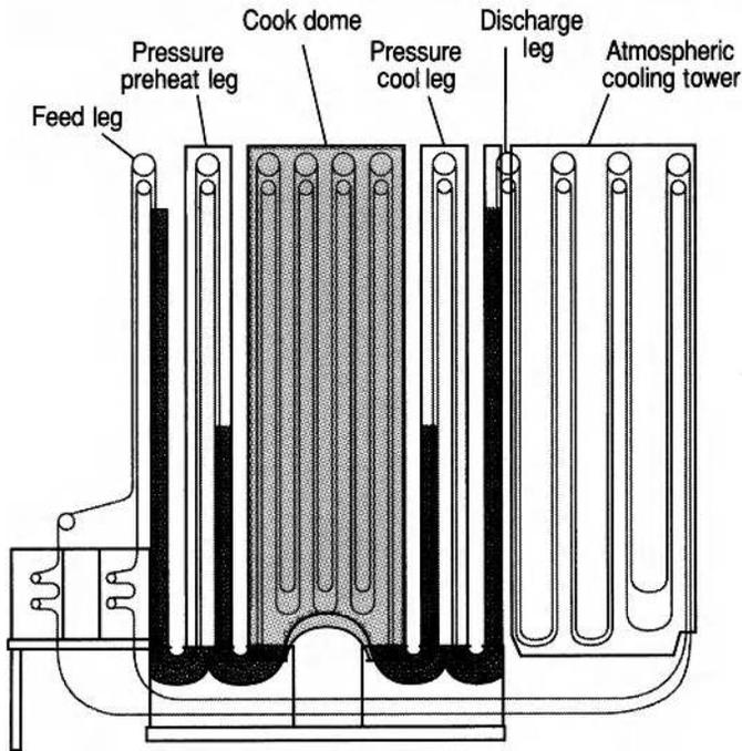
**Fig. 2.5** Hydrostatic cooker-cooler for processing food cans. (Courtesy of JBT FoodTech, formerly known as FMC FoodTech.)
