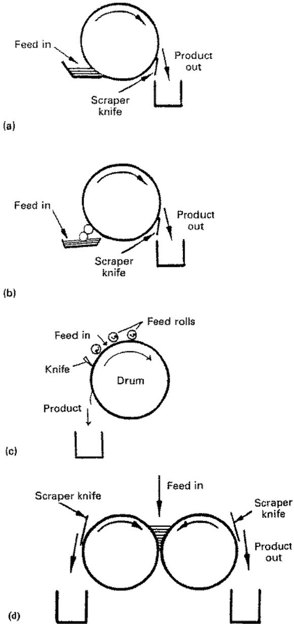
**Fig. 3.14** Different designs of drum driers: (a) single drum with dip feed, (b) single drum with unheated roller feed, (c) single drum with multiroller feed (d) double drum; adapted from [26] with permission.
