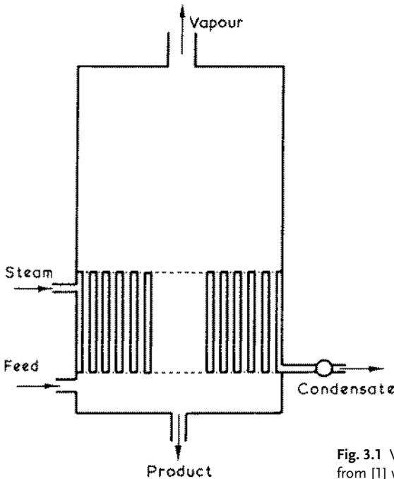
Fig. 3.1 Vertical short tube evaporator; from [1] with permission of the authors.
