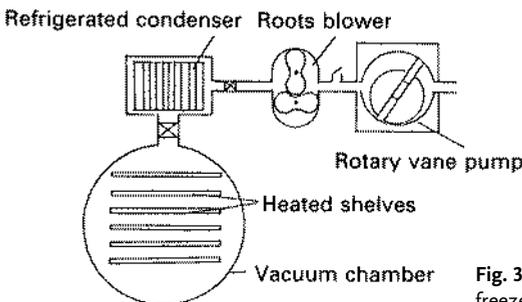
**Fig. 3.9** Main components of a batch freeze drier; from [26] with permission.
