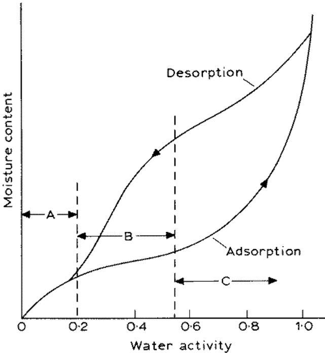
Fig. 3.16 Adsorption and desorption isotherms showing hysteresis; from [1].
