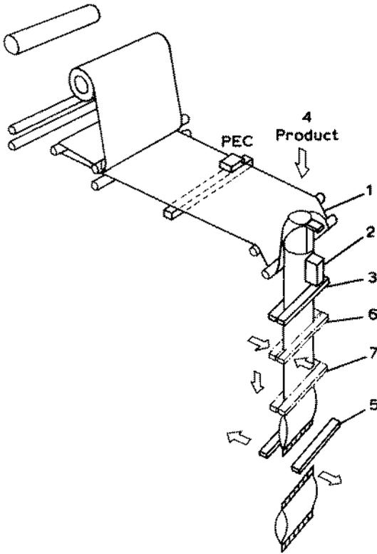
**Fig. 9.2** Vertical form-fill-seal machine for pillow packs. 1. Film from reel made into a tube over forming shoulder. 2. Longitudinal seal made. 3. Bottom of tube closed by heat crimped jaws which move downwards drawing film from reel. 4. Predetermined quantity of product falls through collar into pouch. 5.
