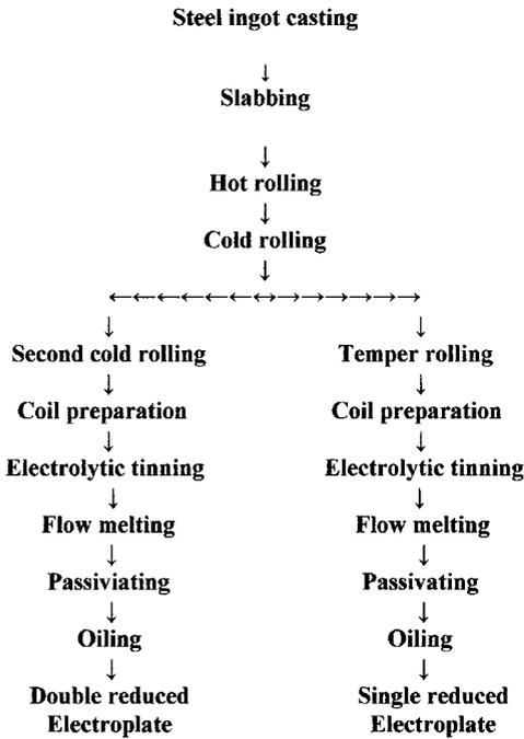
Fig. 9.6 Stages in the manufacture of tinplate.
