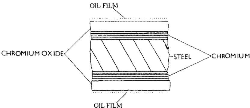
Fig. 9.7 Structure of ECCS plate (tin-free steel).
