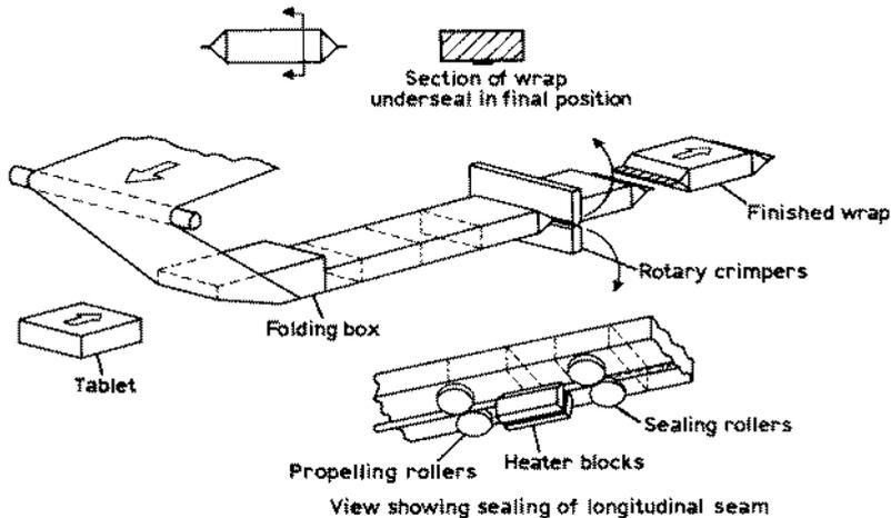
**Fig. 9.4** Horizontal form-fill-seal machine for pillow packs. Film is drawn from reel and formed into horizontal tube around product with continuous seal underneath formed by heater blocks and crimping rollers. Then, rotary heaters make the crimped end seals and cut-off produces individual packs. Adapted from [16] with permission.
