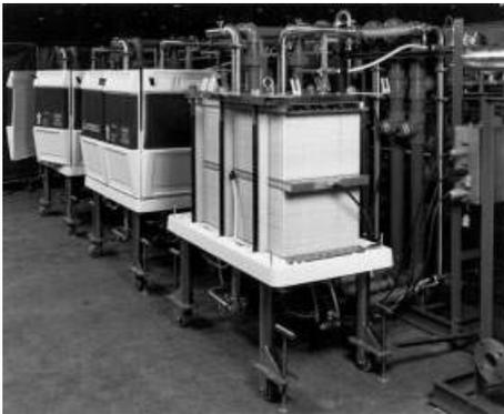
**Fig. 14.35** Electro dialysis membrane stacks; with permission of Ionics Inc.
