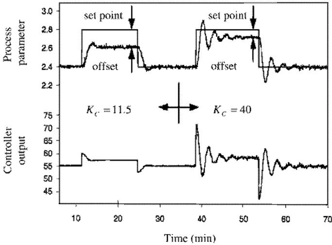
Fig. 11.3 P-controller with two different  $K_c$  values; from [6].
