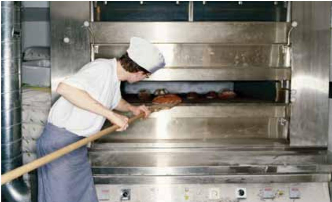
**Dual Baking** Deck ovens are used in high-volume baking to cook a variety of products at once. *Where would you most likely find deck ovens?*
