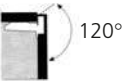
CONCEALED HINGE for standard cabinet lay-on doors. 120° opening angle with spring closing mecha- nism. Similar hinges for 100°, 107° and 170° opening
