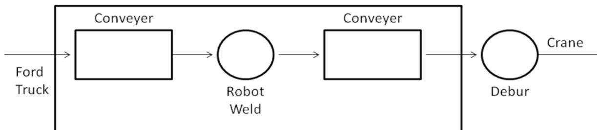
**Figure 3.3** Automated Welding System Detailed Area for Simulation
