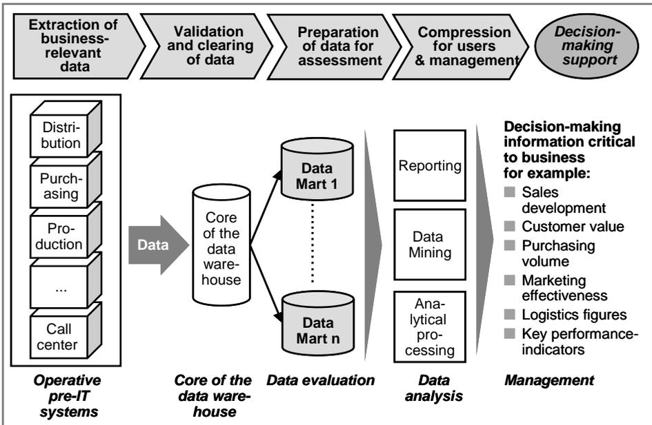
Figure 1.7: Typical architecture of a data warehouse; Source: A.T. Kearney
