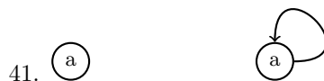
Figure 1: The smallest directed graphs: V = \{a\} with E = \emptyset and E = \{(a, a)\}
