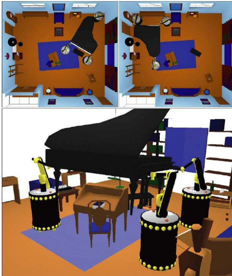
Figure 1.5: Using mobile robots to move a piano [244].
