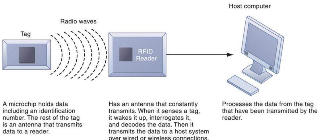
RFID uses low-powered radio transmitters to read data stored in a tag at distances ranging from 1 inch to 100 feet. The reader captures the data from the tag and sends them over a network to a host computer for processing.
