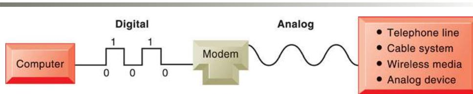
A modem is a device that translates digital signals into analog form (and vice versa) so that computers can transmit data over analog networks such as telephone and cable networks.
