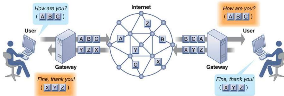
An VoIP phone call digitizes and breaks up a voice message into data packets that may travel along different routes before being reassembled at the final destination. A processor nearest the call's destination, called a gateway, arranges the packets in the proper order and directs them to the telephone number of the receiver or the IP address of the receiving computer.
