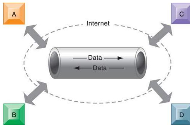
This VPN is a private network of computers linked using a secure “tunnel” connection over the Internet. It protects data transmitted over the public Internet by encoding the data and “wrapping” them within the Internet Protocol (IP). By adding a wrapper around a network message to hide its content, organizations can create a private connection that travels through the public Internet.
