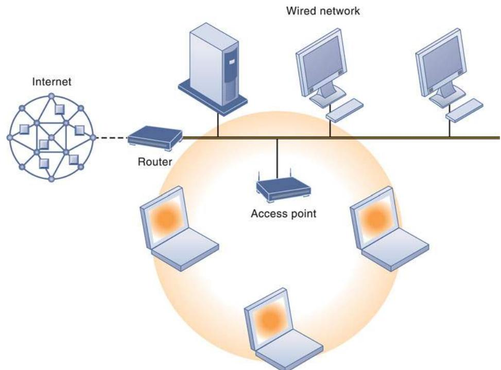
Mobile laptop computers equipped with network interface cards link to the wired LAN by communicating with the access point. The access point uses radio waves to transmit network signals from the wired network to the client adapters, which convert them into data that the mobile device can understand. The client adapter then transmits the data from the mobile device back to the access point, which forwards the data to the wired network.
