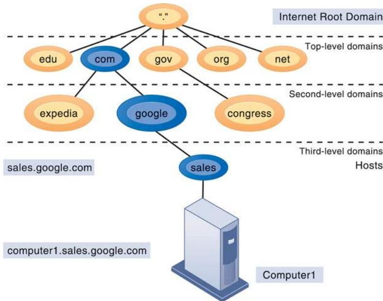
Domain Name System is a hierarchical system with a root domain, top-level domains, second-level domains, and host computers at the third level.
