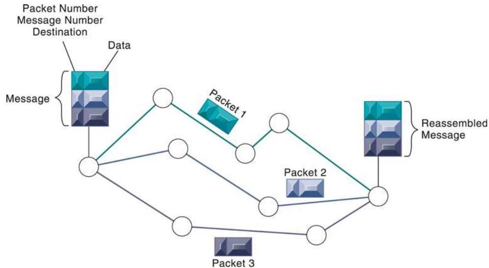
Data are grouped into small packets, which are transmitted independently over various communication channels and reassembled at their final destination.
