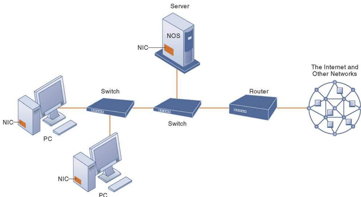
Illustrated here is a very simple computer network, consisting of computers, a network operating system residing on a dedicated server computer, cable (wiring) connecting the devices, network interface cards (NICs), switches, and a router.
