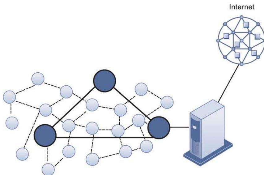
The small circles represent lower-level nodes and the larger circles represent high-end nodes. Lower-level nodes forward data to each other or to higher-level nodes, which transmit data more rapidly and speed up network performance.
