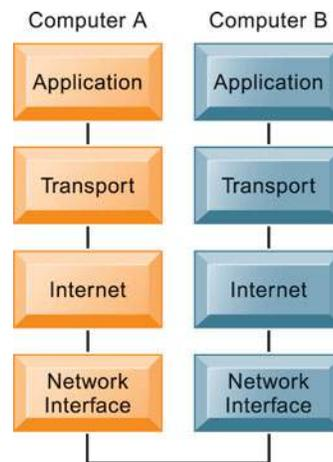
This figure illustrates the four layers of the TCP/IP reference model for communications
