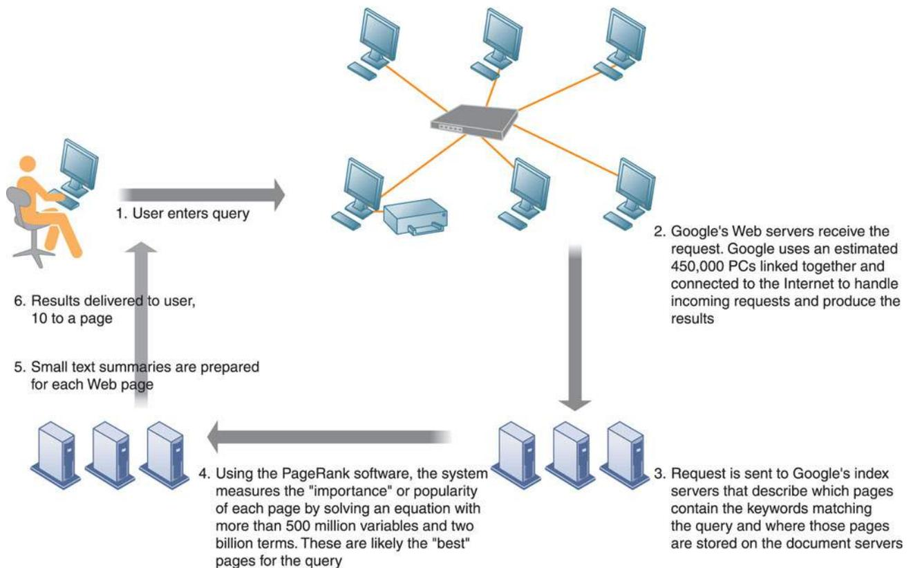
The Google search engine is continuously crawling the Web, indexing the content of each page, calculating its popularity, and storing the pages so that it can respond quickly to user requests to see a page. The entire process takes about one-half second.
