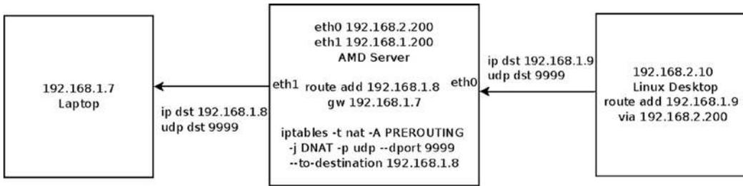
**Figure 9-3.** A simple setup with a DNAT rule
