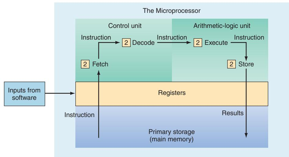
**Figure TG1.5** How the CPU works.
