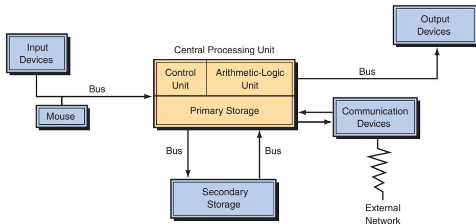
**Figure TG1.1** Components of computer hardware. A bus is a connecting channel.
