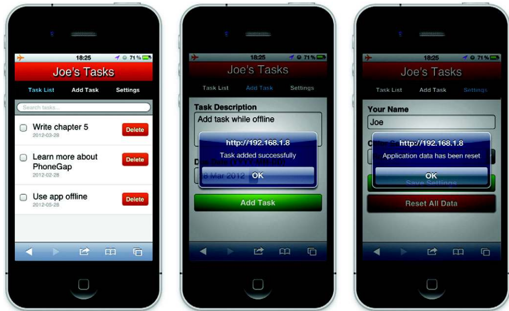
Figure 5.7 My Tasks application running offline. You'll notice the airplane icon in the top left indicating that the phone has no network access. You may also notice that the jazzy font we used in the heading is no longer showing; this font was loaded from the Google Font API, which isn't available when you're offline.
