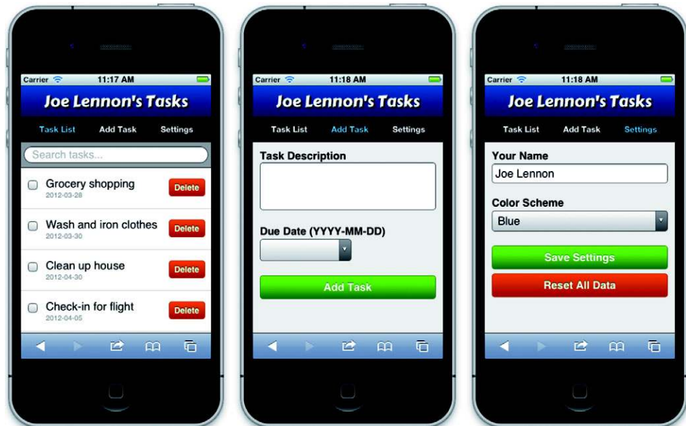
Figure 5.1 The three main views of the My Tasks application: Task List, Add Task, and Settings. To select a view, the application includes a navigation bar near the top.
