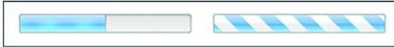
Figure 1.3 The left-hand progress bar is an example of a determinate progress bar. In this example, the value of the bar is set to 50 percent, and the appearance of the bar reflects this because it's half filled. The right-hand progress bar is an indeterminate bar and doesn't have a value. It displays an animated full bar to indicate that something's happening, but the percentage complete isn't known.
