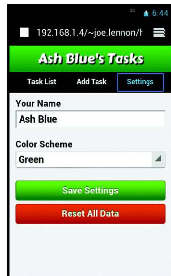
Figure 1.13 In chapter 5, you'll learn how to use the localStorage interface to persist user settings in a mobile task-management application.
