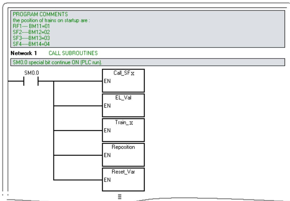
Figure 7.12: The main part of the program (In real there are 3 different Call\_SFz and four Train\_X routines).
