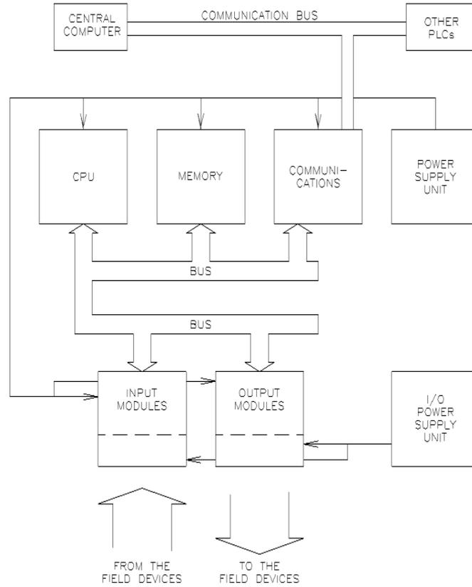
**Figure 7.1:** PLC's block diagram and its interconnections.
