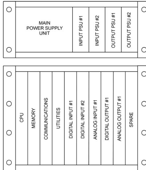
**Figure 7.3:** Typical outline of a modular PLC.
