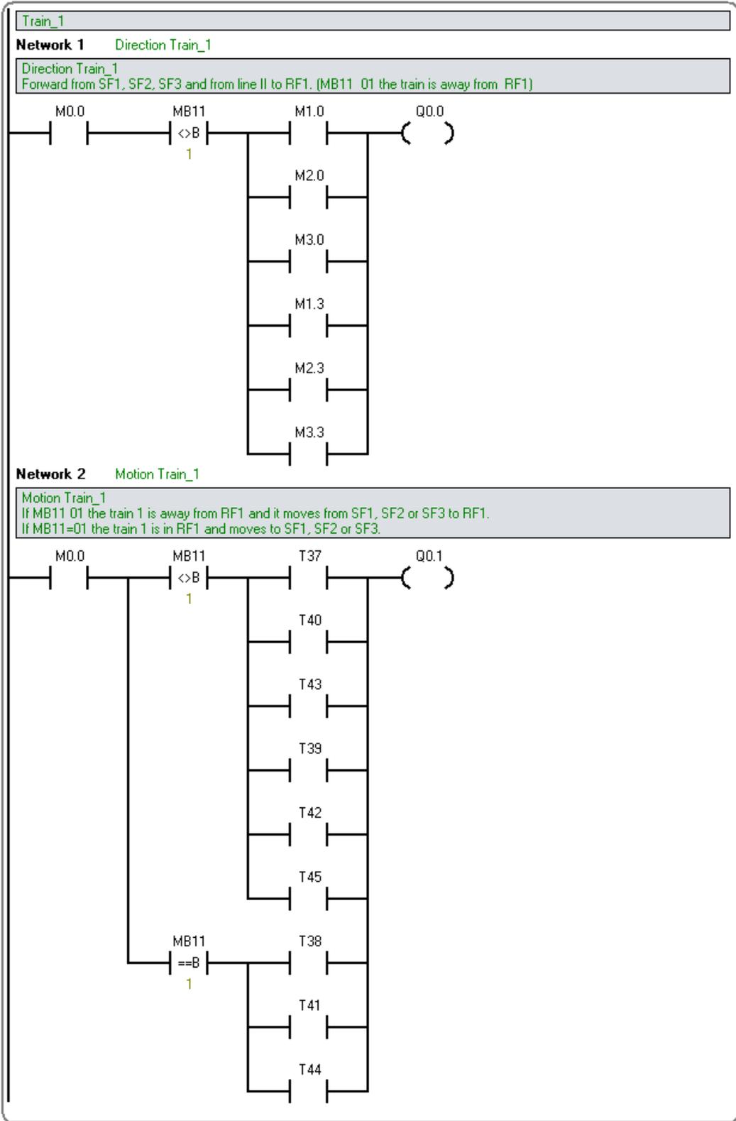
Figure 7.14: The Train\_1 subroutine. The rest derives by the cyclic rotation of the indices.
