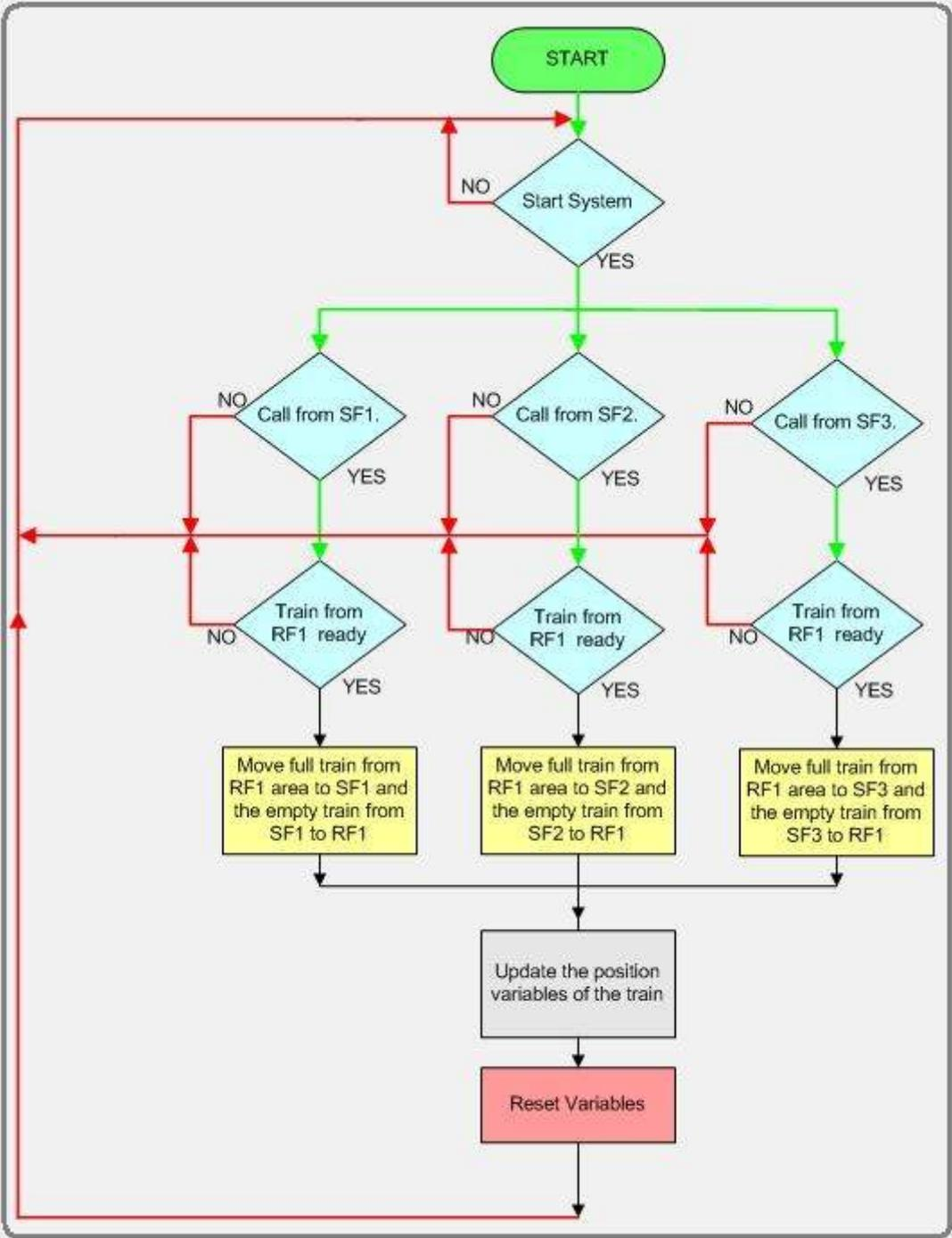
Figure 7.11: The block diagram of the application software.
