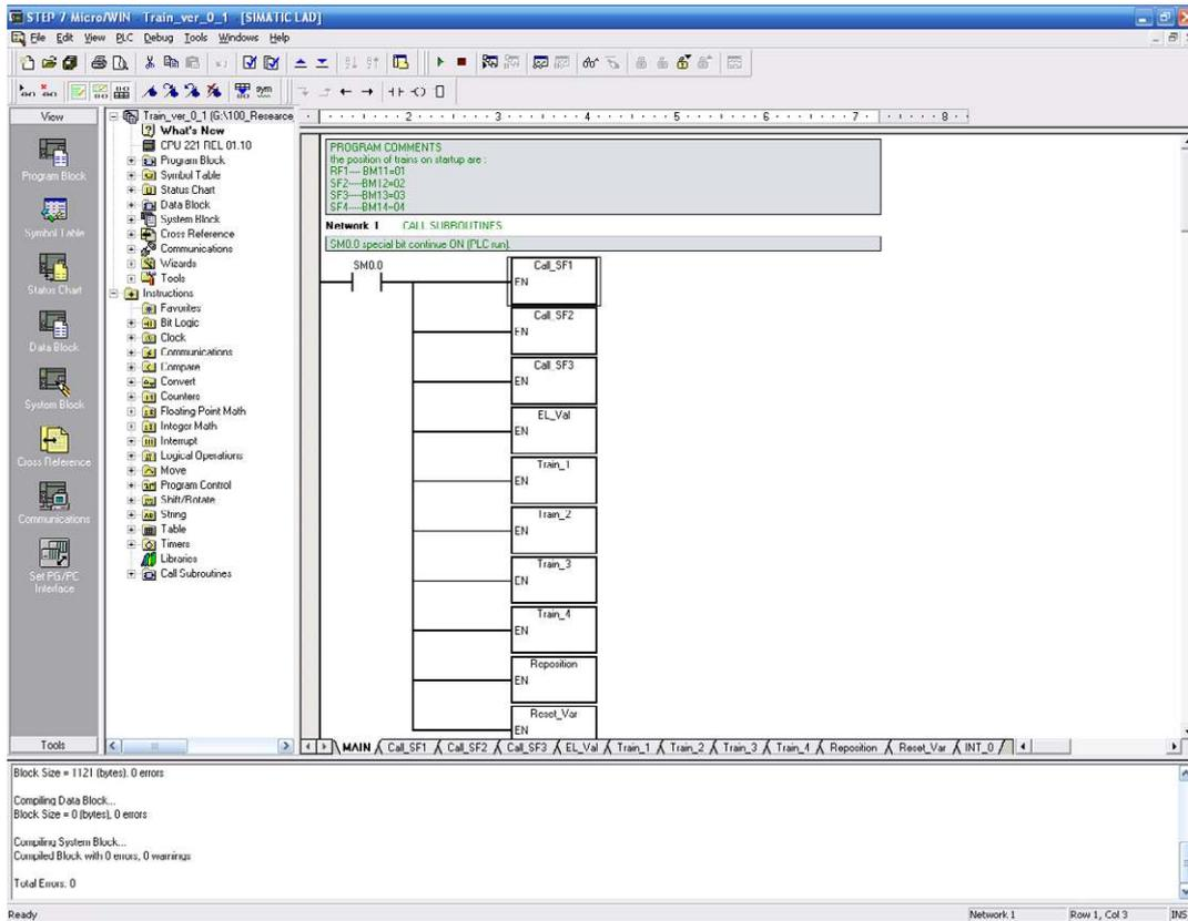
Figure 7.10: The V4.0 STEP 7 MicroWIN programming environment.
