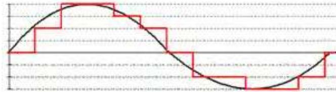
**Figure 5.3:** Continuous (black line) and discrete (red line) value sine-wave signal.
