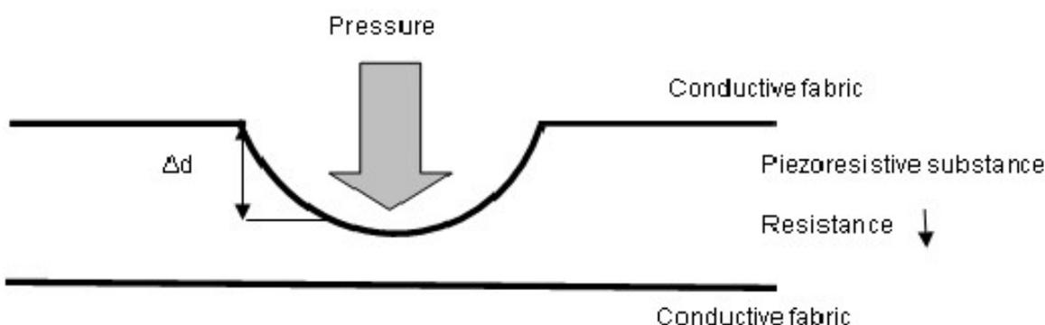
**Figure 3.5:** Principles of piezoresistive sensor (Jeong 2010, p. 89).
