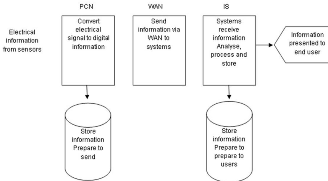
Figure 3.6: End-to-end process flow (Lam 2009, p. 205).
