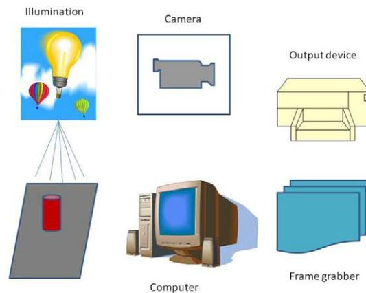
**Figure 9** Components of an image processing system.
