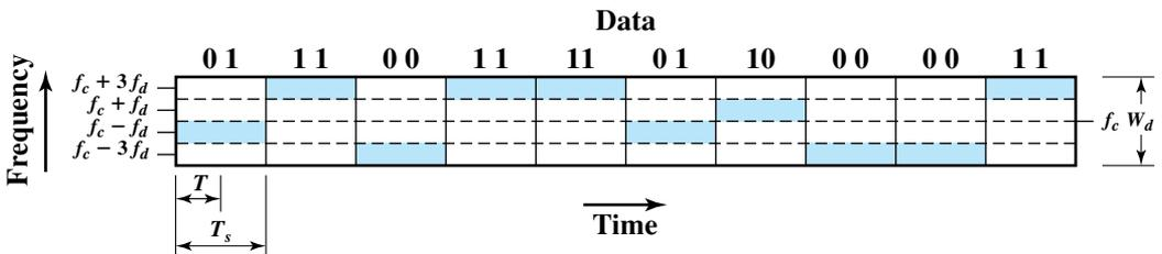
Figure 5.9 MFSK Frequency Use ( $M = 4$ )
