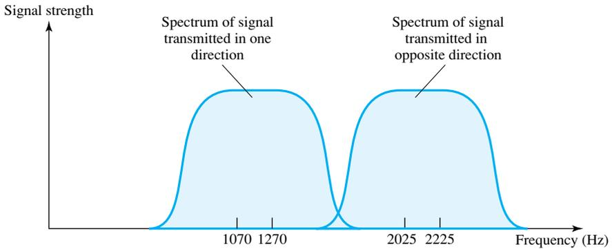
**Figure 5.8** Full-Duplex FSK Transmission on a Voice-Grade Line
