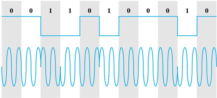
**Figure 5.10** Differential Phase-Shift Keying (DPSK)
