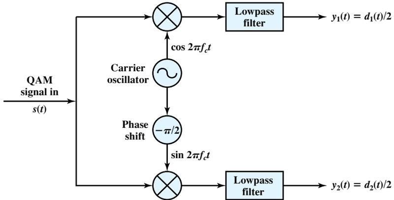
Figure 5.27 QAM Demodulator
