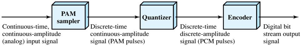
Figure 5.17 PCM Block Diagram
