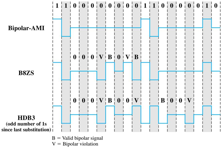
**Figure 5.6** Encoding Rules for B8ZS and HDB3
