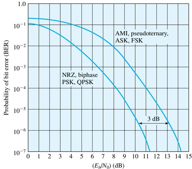
**Figure 5.4** Theoretical Bit Error Rate for Various Encoding Schemes
