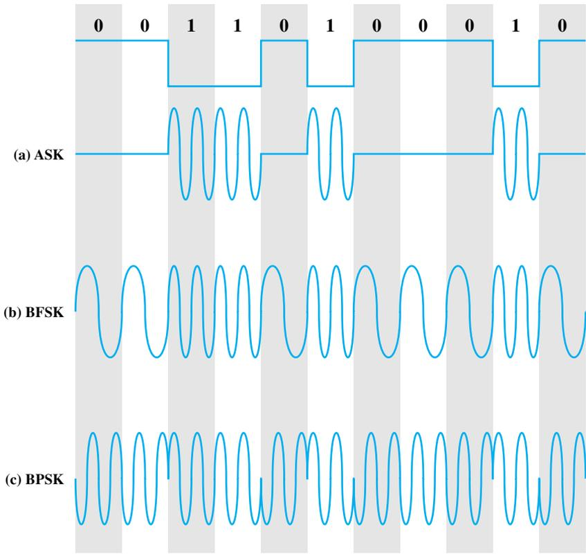
**Figure 5.7** Modulation of Analog Signals for Digital Data
