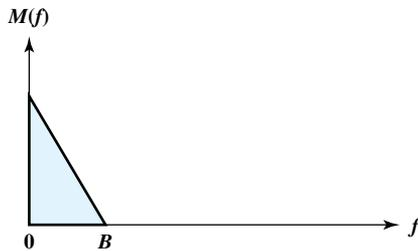
(a) Spectrum of modulating signal
