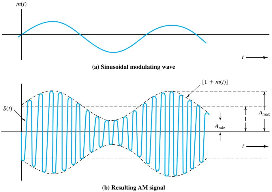
Figure 5.22 Amplitude Modulation
