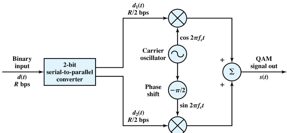
Figure 5.14 QAM Modulator
