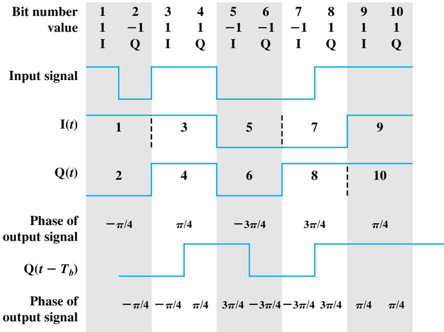
**Figure 5.12** Example of QPSK and OQPSK Waveforms
