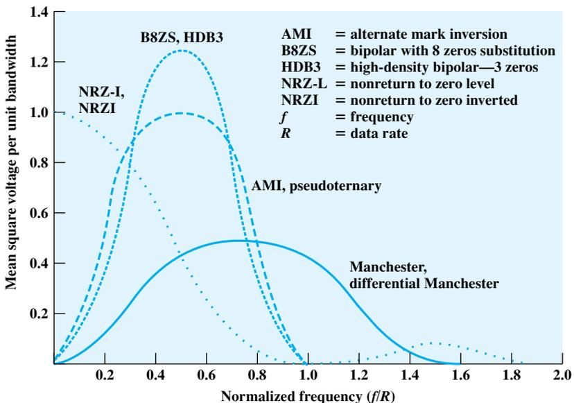
Figure 5.3 Spectral Density of Various Signal Encoding Schemes
