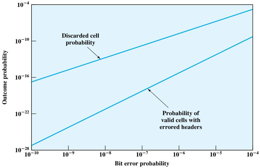
Figure 11.7 Impact of Random Bit Errors on HEC Performance
