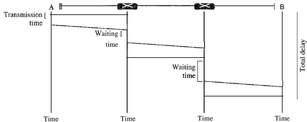
The packet travels through two switches. There are three transmission times ( $3T$ ), three propagation delays (slopes  $3\tau$  of the lines), and two waiting times ( $w_1 + w_2$ ). We ignore the processing time in each switch. The total delay is
