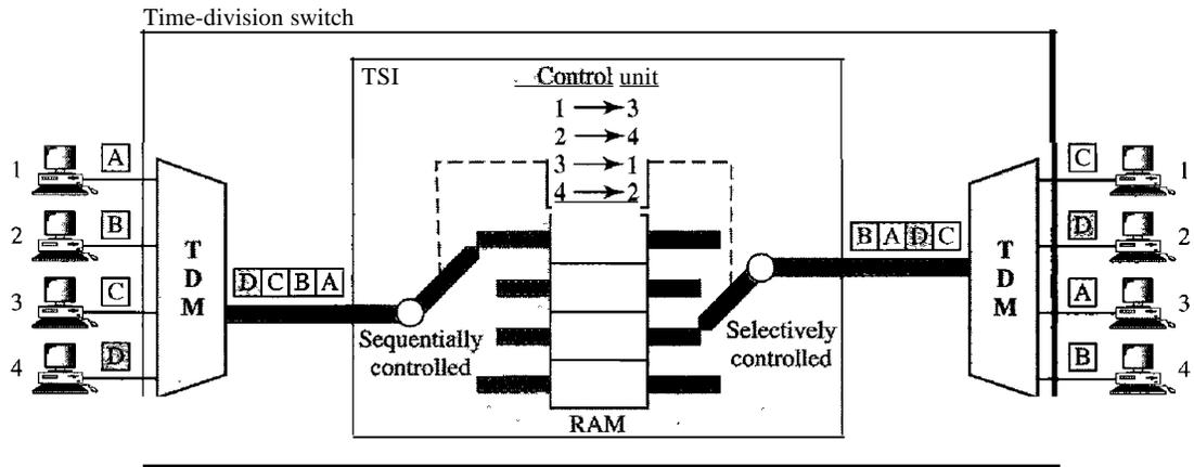
The figure combines a TDM multiplexer, a TDM demultiplexer, and a TSI consisting of random access memory (RAM) with several memory locations. The size of each location is the same as the size of a single time slot. The number of locations is the same as the number of inputs (in most cases, the numbers of inputs and outputs are equal). The RAM fills up with incoming data from time slots in the order received. Slots are then sent out in an order based on the decisions of a control unit.
