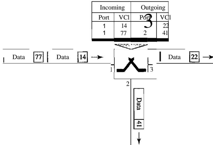
Figure 8.13 Source-to-destination data transfer in a virtual-circuit network
