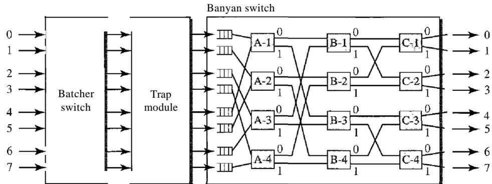
**Batcher-Banyan Switch** The problem with the banyan switch is the possibility of internal collision even when two packets are not heading for the same output port. We can solve this problem by sorting the arriving packets based on their destination port.
