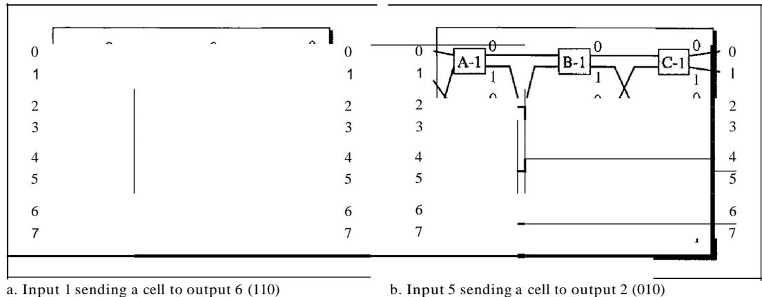
a. Input 1 sending a cell to output 6 (110)
