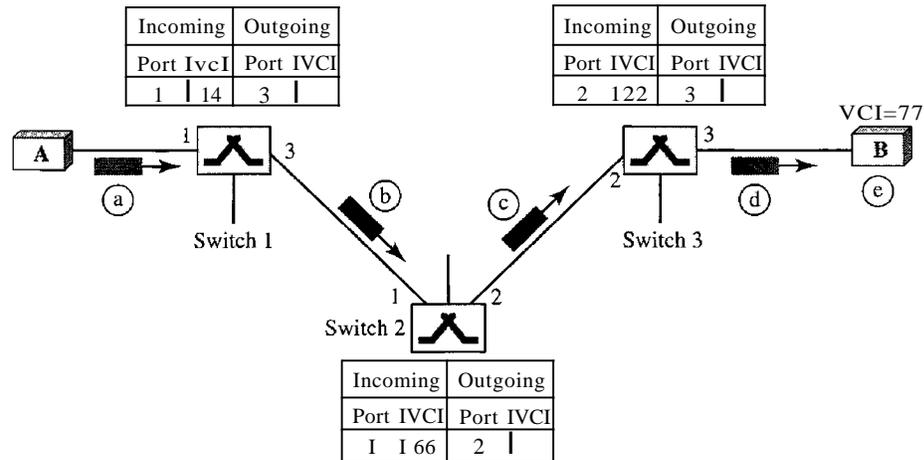
this virtual circuit, but it is only able to fill three of the four columns. The switch assigns the incoming port (1) and chooses an available incoming VCI (14) and the outgoing port (3). It does not yet know the outgoing VCI, which will be found during the acknowledgment step. The switch then forwards the frame through port 3 to switch 2.
