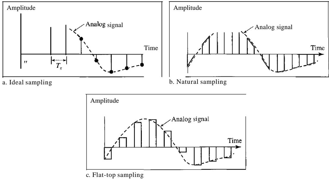
According to the Nyquist theorem, the sampling rate must be at least 2 times the highest frequency contained in the signal.
