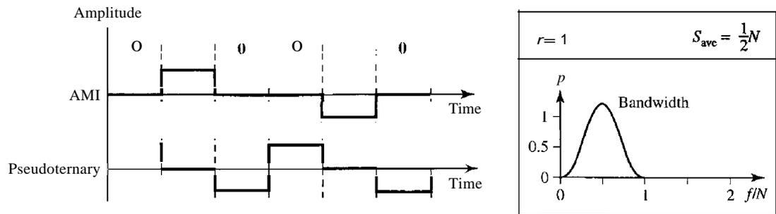
The bipolar scheme was developed as an alternative to NRZ. The bipolar scheme has the same signal rate as NRZ, but there is no DC component. The NRZ scheme has most of its energy concentrated near zero frequency, which makes it unsuitable for transmission over channels with poor performance around this frequency. The concentration of the energy in bipolar encoding is around frequency  $N/2$ . Figure 4.9 shows the typical energy concentration for a bipolar scheme.
