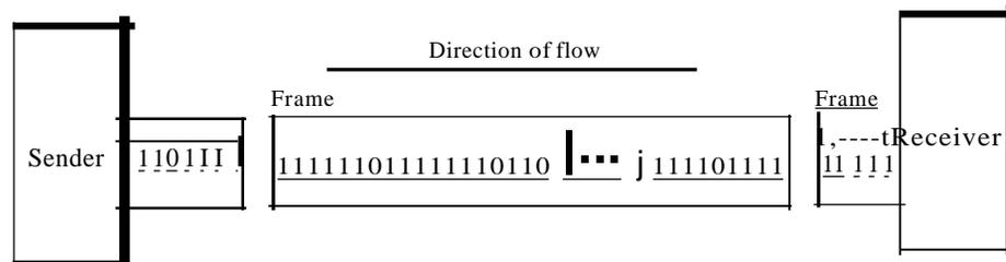
Without gaps and start and stop bits, there is no built-in mechanism to help the receiving device adjust its bit synchronization midstream. Timing becomes very important, therefore, because the accuracy of the received information is completely dependent on the ability of the receiving device to keep an accurate count of the bits as they come in.
