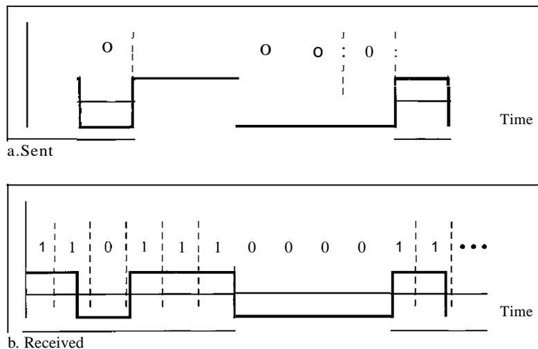
A self-synchronizing digital signal includes timing information in the data being transmitted. This can be achieved if there are transitions in the signal that alert the receiver to the beginning, middle, or end of the pulse. If the receiver's clock is out of synchronization, these points can reset the clock.
