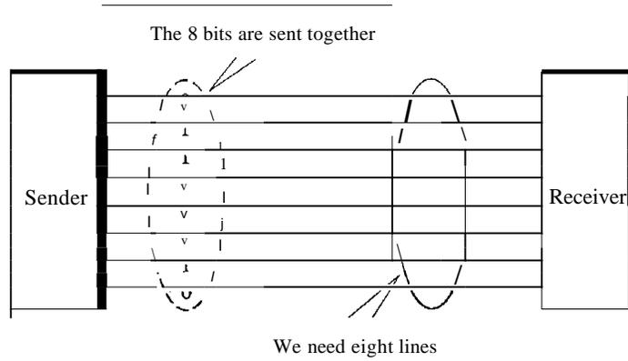
But there is a significant disadvantage: cost. Parallel transmission requires  $n$  communication lines (wires in the example) just to transmit the data stream. Because this is expensive, parallel transmission is usually limited to short distances.
