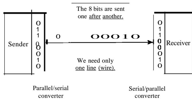
The advantage of serial over parallel transmission is that with only one communication channel, serial transmission reduces the cost of transmission over parallel by roughly a factor of  $n$ .
