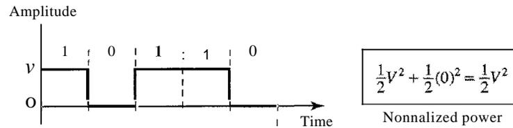
Compared with its polar counterpart (see the next section), this scheme is very costly. As we will see shortly, the normalized power (power needed to send 1 bit per unit line resistance) is double that for polar NRZ. For this reason, this scheme is normally not used in data communications today.
