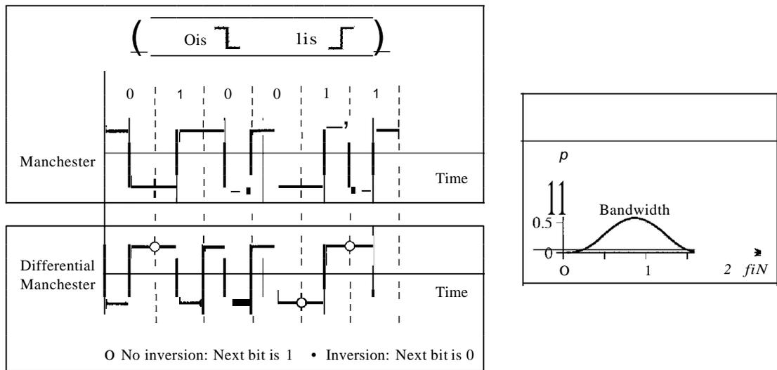
In Manchester and differential Manchester encoding, the transition at the middle of the bit is used for synchronization.
