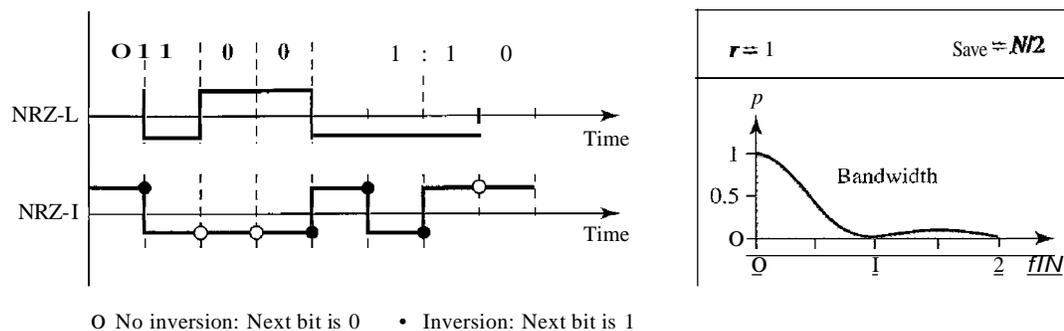
**In NRZ-L** the level of the voltage determines the value of the bit. **In NRZ-I** the inversion or the lack of inversion determines the value of the bit.
