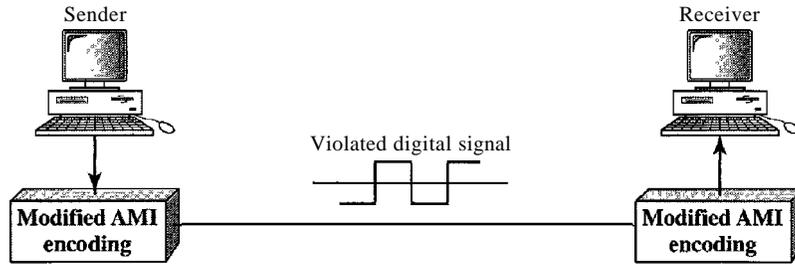
OOOVBOVB. The V in the sequence denotes *violation*; this is a nonzero voltage that breaks an AMI rule of encoding (opposite polarity from the previous). The B in the sequence denotes *bipolm*; which means a nonzero level voltage in accordance with the AMI rule. There are two cases, as shown in Figure 4.19.
