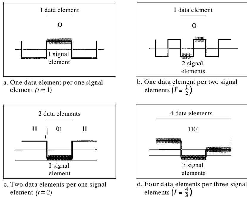
In part a of the figure, one data element is carried by one signal element ( $r = 1$ ). In part b of the figure, we need two signal elements (two transitions) to carry each data
