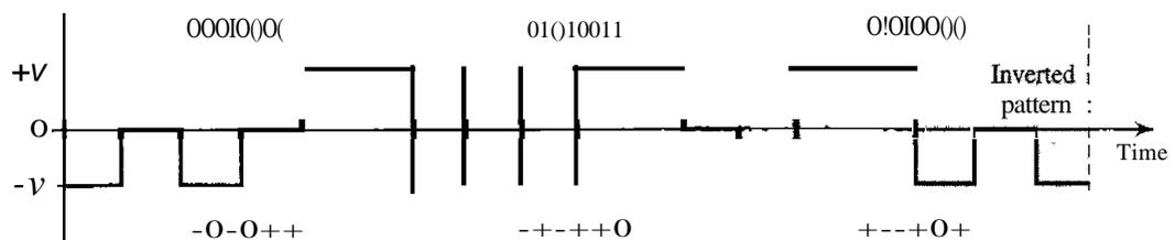
The average signal rate of the scheme is theoretically  $S_{ave} = \frac{1}{2} \times N \times \frac{6}{8}$ ; in practice the minimum bandwidth is very close to  $6N/8$ .
