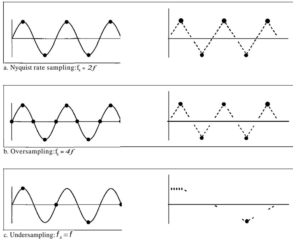
It can be seen that sampling at the Nyquist rate can create a good approximation of the original sine wave (part a). Oversampling in part b can also create the same approximation, but it is redundant and unnecessary. Sampling below the Nyquist rate (part c) does not produce a signal that looks like the original sine wave.
