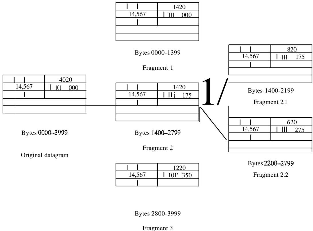
The figure also shows what happens if a fragment itself is fragmented. In this case the value of the offset field is always relative to the original datagram. For example, in the figure, the second fragment is itself fragmented later to two fragments of 800 bytes and 600 bytes, but the offset shows the relative position of the fragments to the original data.
