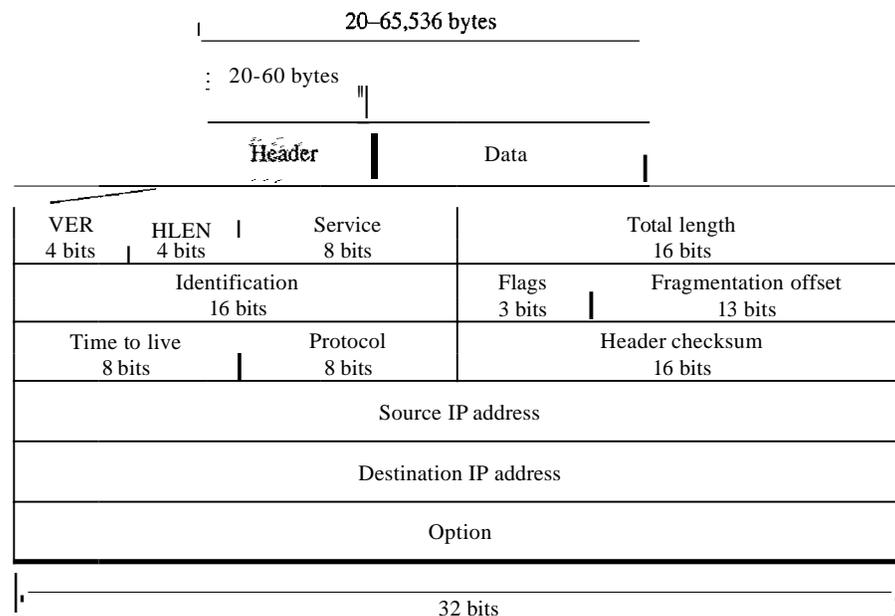
A datagram is a variable-length packet consisting of two parts: header and data. The header is 20 to 60 bytes in length and contains information essential to routing and
