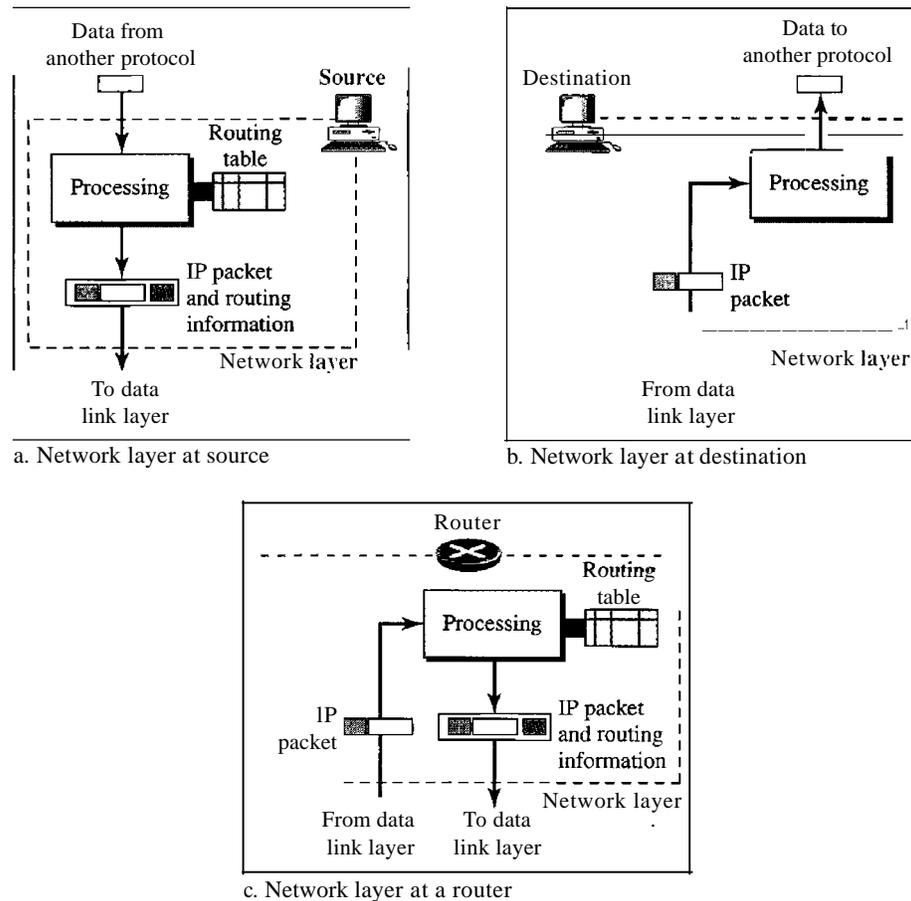
The network layer at the switch or router is responsible for routing the packet. When a packet arrives, the router or switch consults its routing table and finds the interface from which the packet must be sent. The packet, after some changes in the header, with the routing information is passed to the data link layer again.
