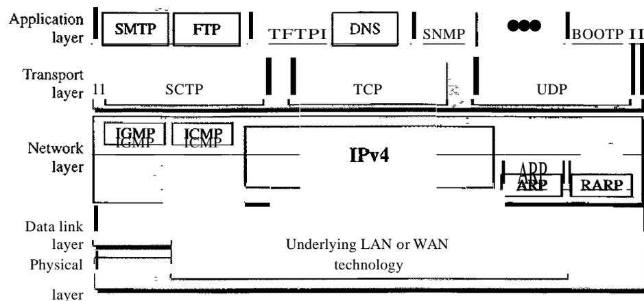
IPv4 is an unreliable and connectionless datagram protocol—a best-effort delivery service. The term *best-effort* means that IPv4 provides no error control or flow control (except for error detection on the header). IPv4 assumes the unreliability of the underlying layers and does its best to get a transmission through to its destination, but with no guarantees.
