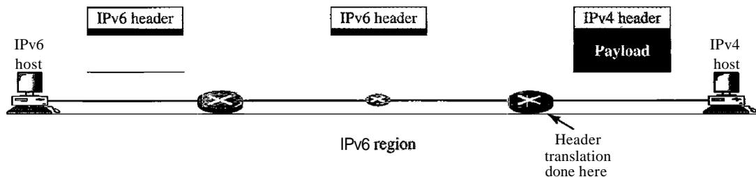
Header translation uses the mapped address to translate an IPv6 address to an IPv4 address. Table 20.11 lists some rules used in transforming an IPv6 packet header to an IPv4 packet header.
