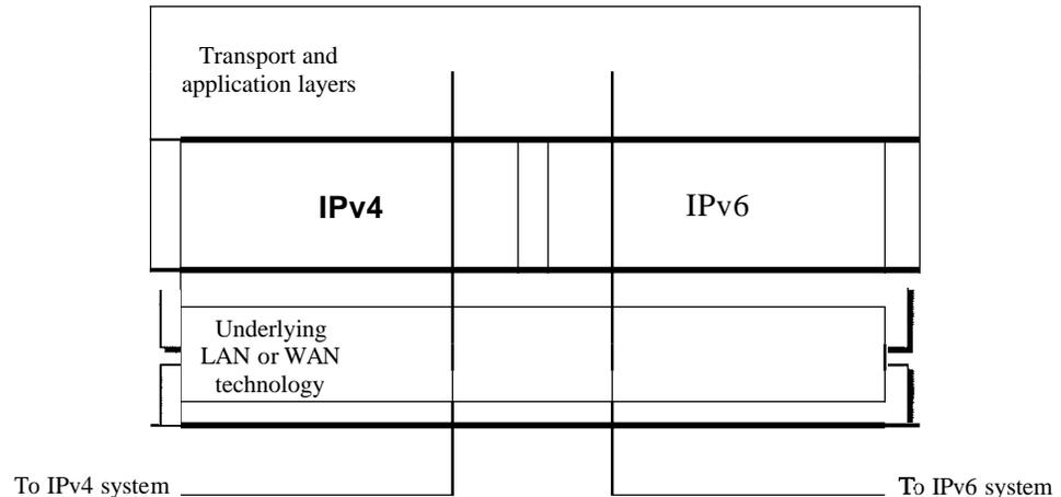
To determine which version to use when sending a packet to a destination, the source host queries the DNS. If the DNS returns an IPv4 address, the source host sends an IPv4 packet. If the DNS returns an IPv6 address, the source host sends an IPv6 packet.
