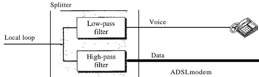
Note that the splitter needs to be installed at the customer's premises, normally by a technician from the telephone company. The voice line can use the existing telephone wiring in the house, but the data line needs to be installed by a professional. All this makes the ADSL line expensive. We will see that there is an alternative technology, Universal ADSL (or ADSL Lite).
