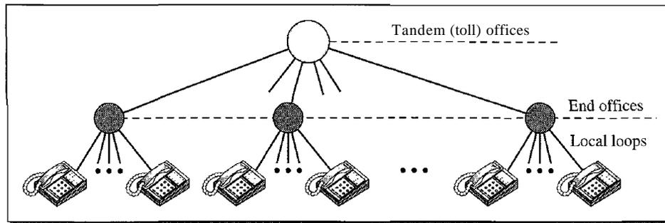
Communication inside a LATA is handled by end switches and tandem switches. A call that can be completed by using only end offices is considered toll-free. A call that has to go through a tandem office (intra-LATA toll office) is charged.
