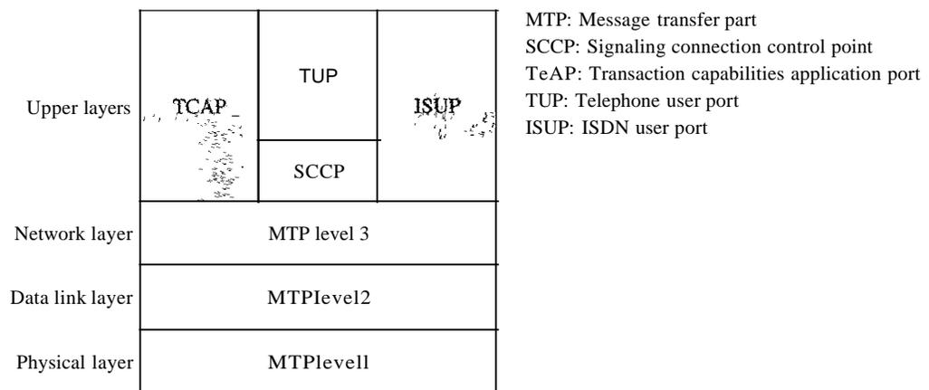
**Physical Layer: MTP Level 1** The physical layer in SS7 called message transport part (MTP) level 1 uses several physical layer specifications such as T-1 (1.544 Mbps) and DCa (64 kbps).
