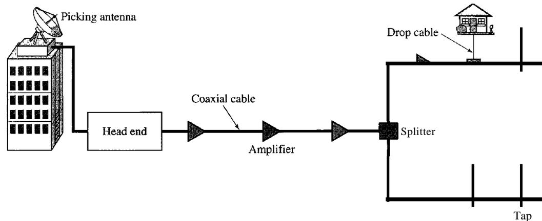
The cable TV office, called the head end, receives video signals from broadcasting stations and feeds the signals into coaxial cables. The signals became weaker and weaker with distance, so amplifiers were installed through the network to renew the signals. There could be up to 35 amplifiers between the head end and the subscriber premises. At the other end, splitters split the cable, and taps and drop cables make the connections to the subscriber premises.
