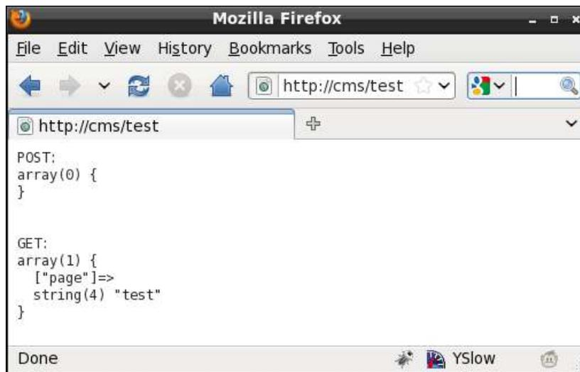
Notice the `GET` array now has the page name, which we can use in the next section to retrieve data from the database.
