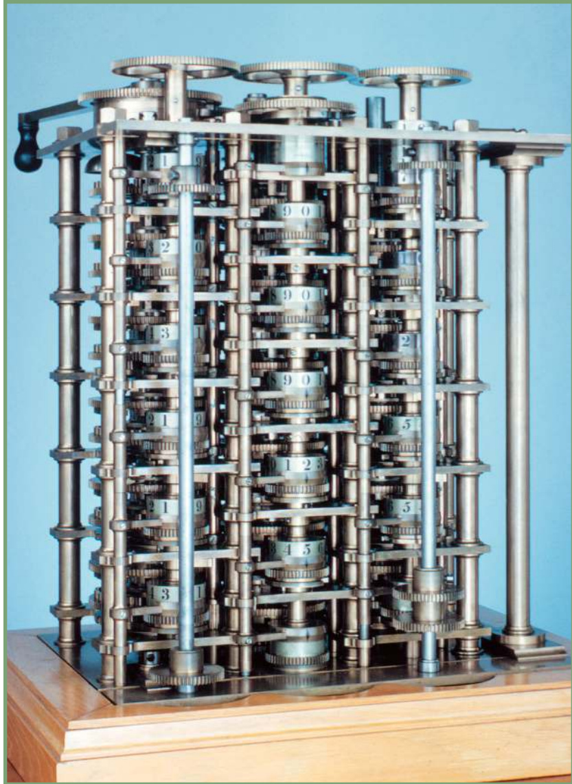
Figure 2.4 Charles Babbage first conceived the idea of an advanced calculating machine to calculate and print mathematical tables in 1812, as a way to eliminate inaccuracies associated with compiling mathematical tables by hand. Difference Engine No. 1 (above) was begun in 1824 and assembled in 1832 by Joseph Clement, a skilled toolmaker and draughtsman. It was a decimal digital machine—the value of a number represented by the positions of toothed wheels marked with decimal numbers.
