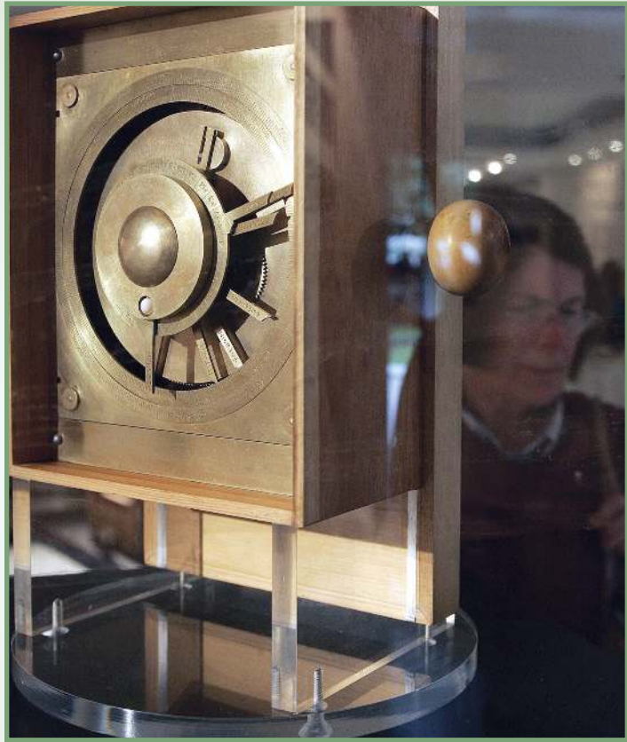
Figure 2.1 A reconstruction of an Antikythera device is shown on display at the Second International Conference on the Ancient Technology in Athens, Greece, in 2005. It consists of at least 29 gears of various sizes that were made to move simultaneously via a handle.
