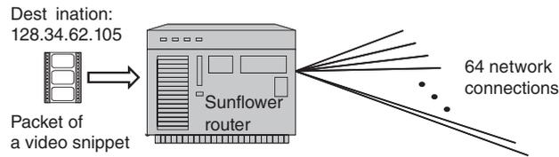
Suppose you are working on a development team that is designing the next generation of a network router for a major technology company. Such devices process information packets, allowing them to move through networks having lots of interconnections. In this case, your team’s job is to design a router, code named “Sunflower,” that can process 64 streams of high-definition video at a time.
