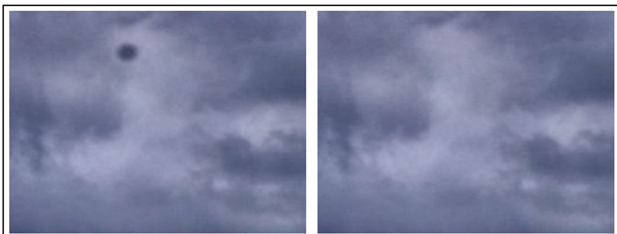
Fig 9.4 on the left is a prominent sensor dust spot. On the right we have the same area fixed using the Healing Brush.
