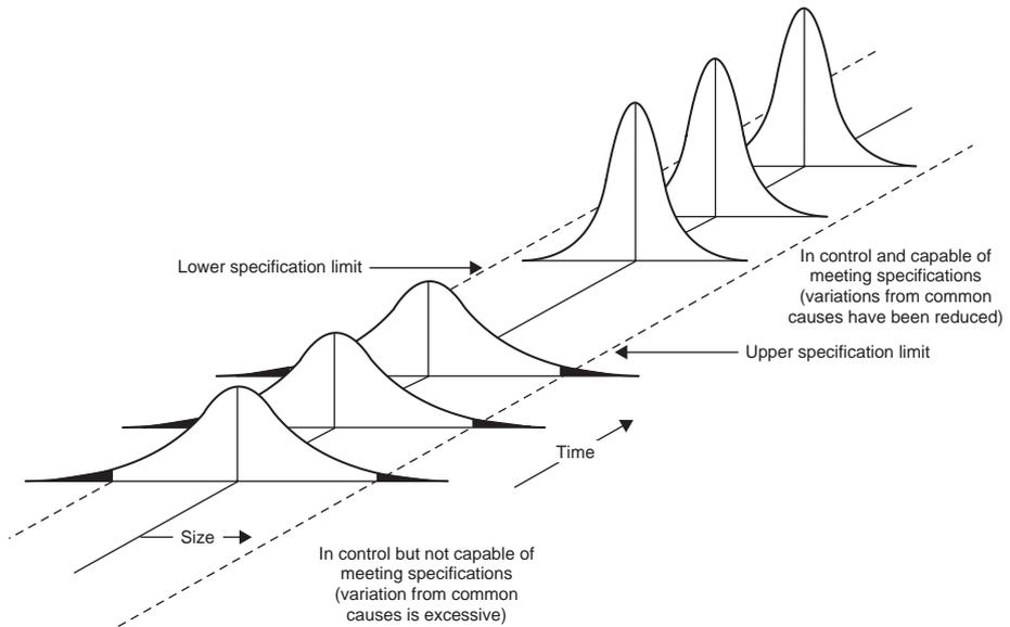
**Figure 2.9** From process control to capable process
