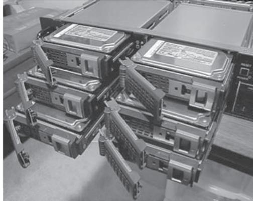
**FIGURE 2-12** A redundant array of inexpensive disks (RAID).
