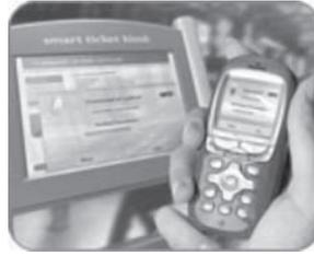
**FIGURE 2-18** Near field communication devices.
